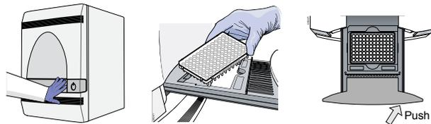
2. Place the calibration plate inside its packaging sleeve. If you plan to perform background and optical calibrations:
