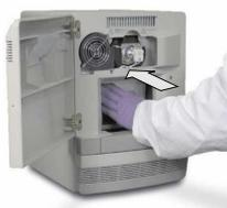
7. Clean the contaminated wells of the sample block using a small volume of deionized water:
