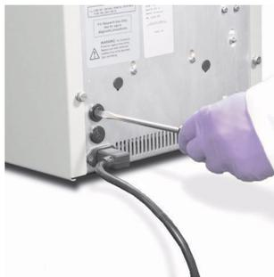
6. Plug in, then power on the instrument.
