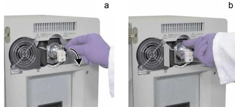
4. Inspect the lamp for signs of failure (carbon typically coats the inside of failed lamps).
