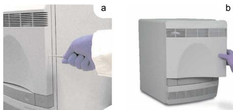
6. Lift the latch, then push the heated cover door to the back of the instrument.
