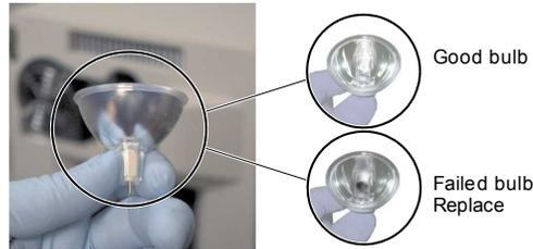
5. Install the new lamp into the instrument:
