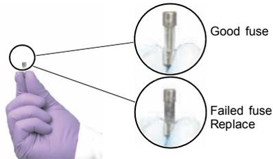
4. Replace each failed fuse with a 12.5 A, 250 V, 5 · 20-mm fuse.
