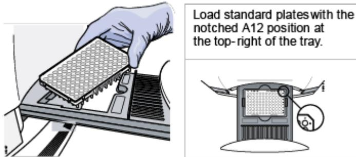
3. Close the tray door. Apply pressure to the right side of the tray door at an angle.
