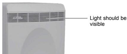
11. If the lamp is illuminated, select **Instrument ▶ Lamp Status/Replacement** in the Real-Time PCR Software, click **Reset Lamp Timer**, then click **OK**.
